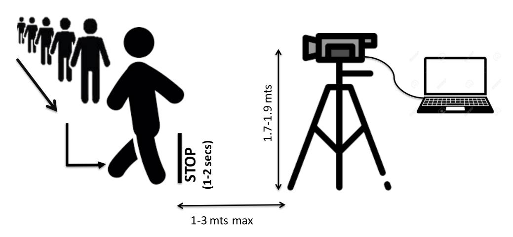
We recommend to set the camera perpendicular to the line. This will allow us to analyze one person at a time. The individual will have to face the camera to be scanned.
